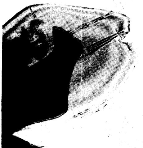
Fig. 16. Deformed platelet aged for 12 hr at 760°C.
