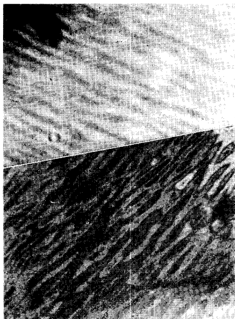
Fig. 6. Thin foil as solution treated, vein structure, \times 20,000 .
