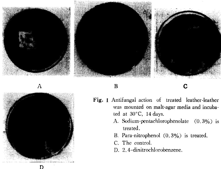
Fig. 1 Antifungal action of treated leather-leather was mounted on malt-agar media and incubated at 30°C, 14 days.
