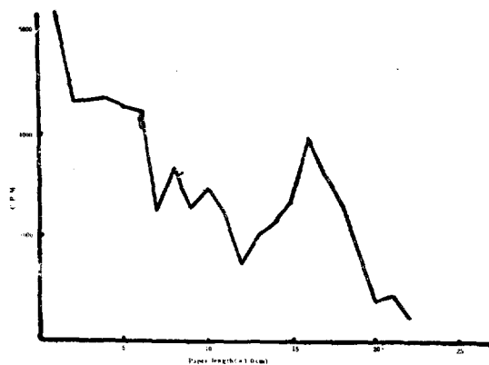
Fig 11. Thickness and activity calibrated radiochromatogram ( \text{CH}_2\text{CICOOH} ). A = (T - Ta)/c + S/c Where C is the activity calibration factor.
