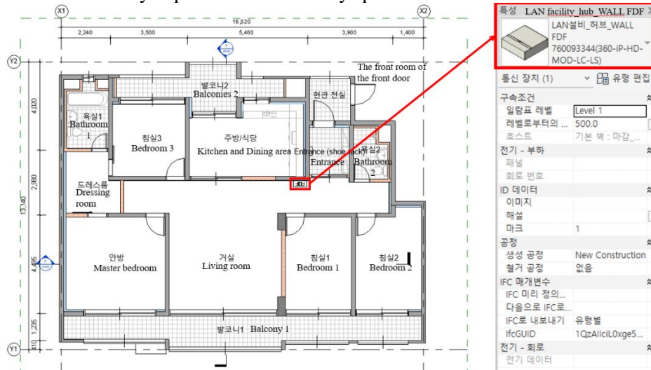
Fig 7. Floor plan and generation junction box library
