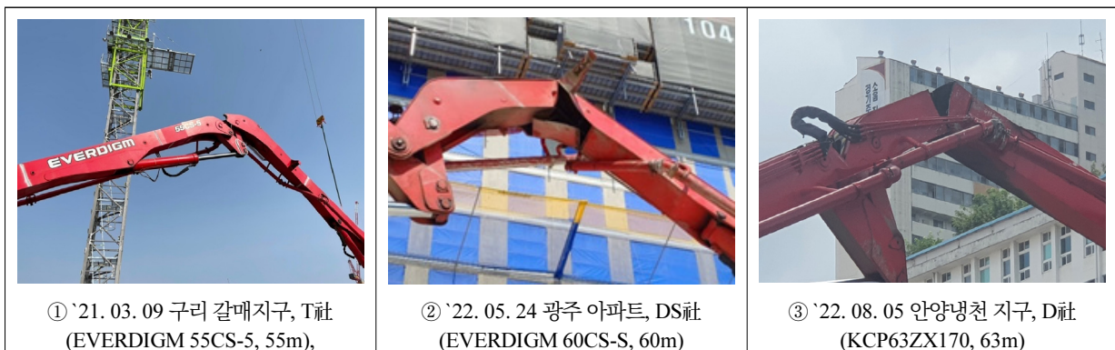
Fig. 1. Current status of concrete pump truck accidents
