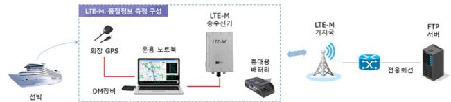
Fig. 4 Configuration of LTE-M. quality measurement
