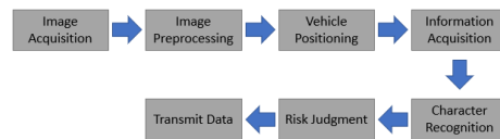
Fig. 7. Car object recognition process
