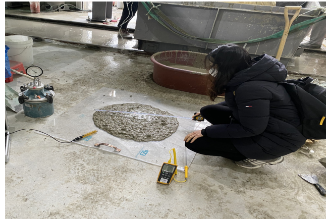
Figure 2. Slump flow and air content test
