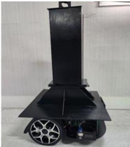
Fig. 1. Illegal Parking Enforcement Robot
