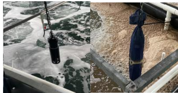
Fig. 2. Water quality sensor
