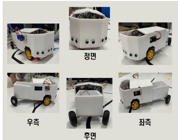
Fig. 4. Transfer Device using Line Tracer
