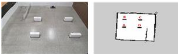
Fig. 3. Virtual environment and Map made with SLAM
