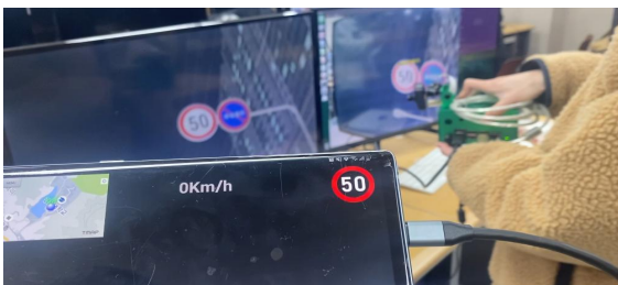
Fig. 4. A display result for traffic sign using object recognition
