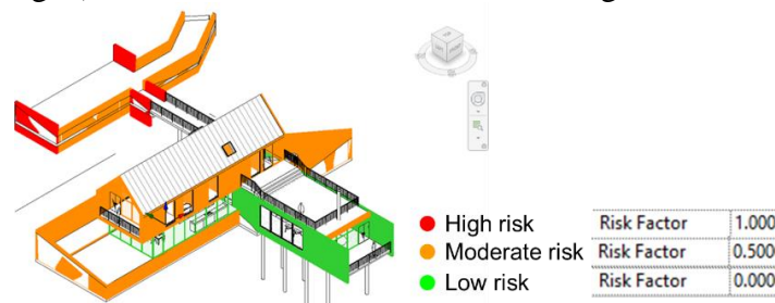
Figure 6. Example of tracking risk factor for walls in Autodesk Revit sample project using the dynamo script (semi-automatic assignment based on the elements' parameters)
