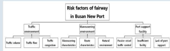
Fig.3 Structure of AHP analysis for risk factors in Busan New Port fairway
