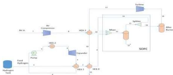
Fig. 1 The Schematic of SOFC integrated system
