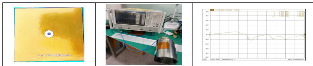
Fig. 3. Fabricated flexible surface wave resonator and return loss
