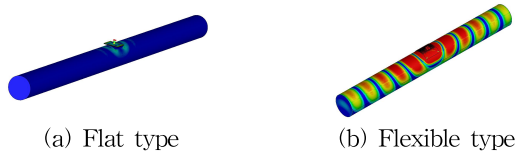
Fig. 1. Comparison of signal transmission EM simulation between planar and flexible resonators in a cylindrical structure
