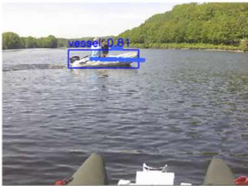
Figure 4. LiDAR-camera sensor fusion result based on the neural network model.
