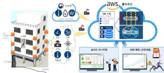
그림 1. Configuration of cloud-based real-time building health monitoring and prediction system
