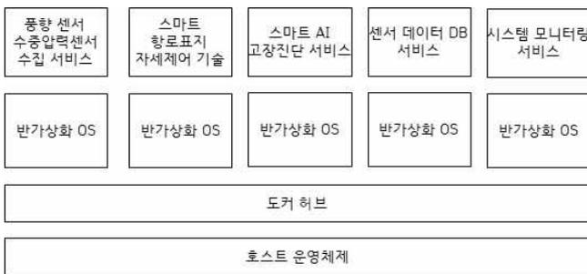
Fig. 1 Docker architecture for smart aids to navigation
