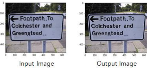
Fig. 2. Sharpening Filter Result
