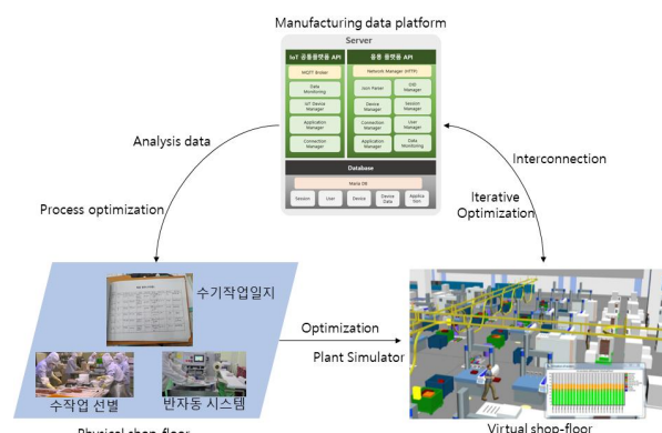
Fig. 2. The virtual factory framework using Plant Simulator
