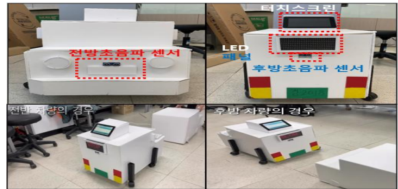
Fig. 4. Front & Real Safety LED Panel for Vehicle
