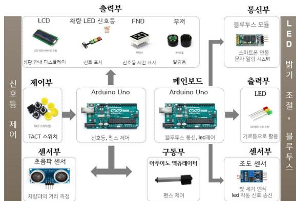
Fig. 1. Diagram of Protective electronic control signal light for children
