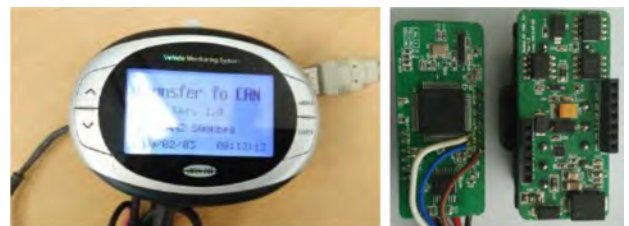
(그림 1) OBDII Device(Left) / OBDII Gender PCB(Right)
