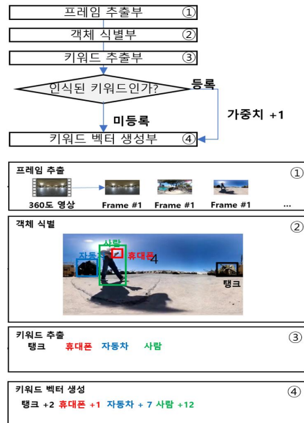
Fig. 4. Advertising Keyword Recognition Process Through Object Recognition
