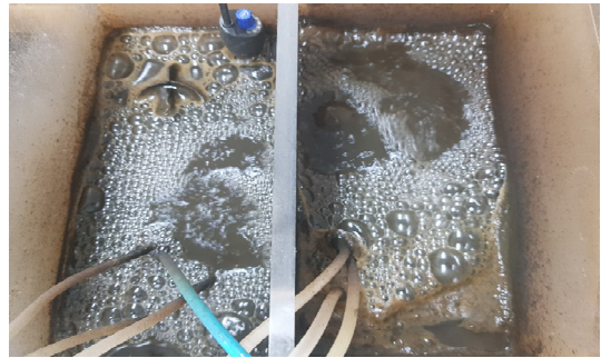
Fig. 2. Bioreactor tank during aeration period.
