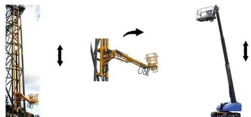
○ guide rail 적용 ○ slewing post 적용 ○ telescopic arm Fig. 1 Optional devices in Service and Access Basket
