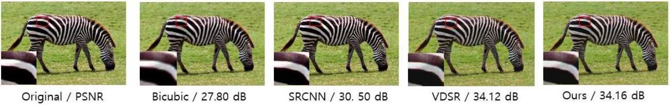
Figure 6. Super resolution results for image zebra with scale factor \times 2 from set14
