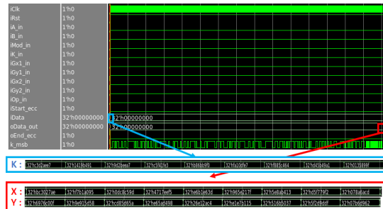
Fig. 3. Simulation results of DF-ECC processor over B-283 Koblitz curve
