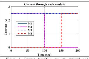
Figure 4. Current transition due to removal and addition of modules
