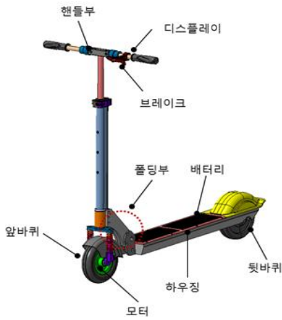
Fig. 1. Electric Kickboard Components
