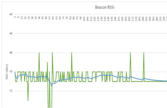
Fig. 2. Kalman filter applied Beacon RSSI Graph
