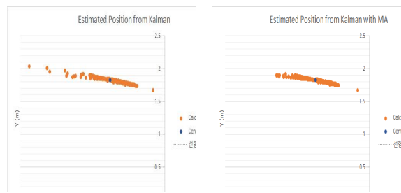
Fig. 4. Positions about Kalman only and Kalman with Moving Average applied
