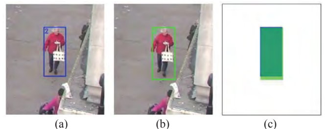
Figure 2. Bounding boxes of a pedestrian in two consecutive frames overlap each other. (a) Bounding box in frame t - 1 (b) Bounding box in frame t (c) Overlapped region
