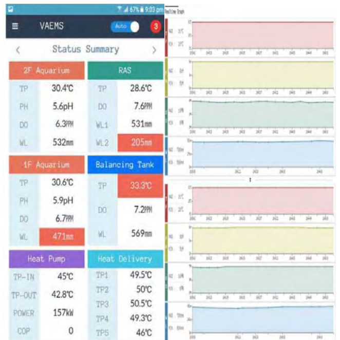
(Figure 4) Heat Pump and Monitoring Control System Mobile app.
