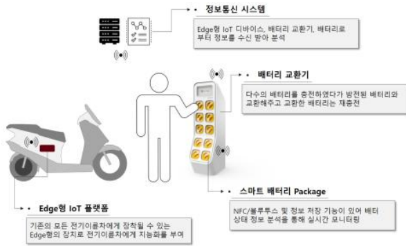
Fig. 1. Battery swapping two-wheeler vehicle system
