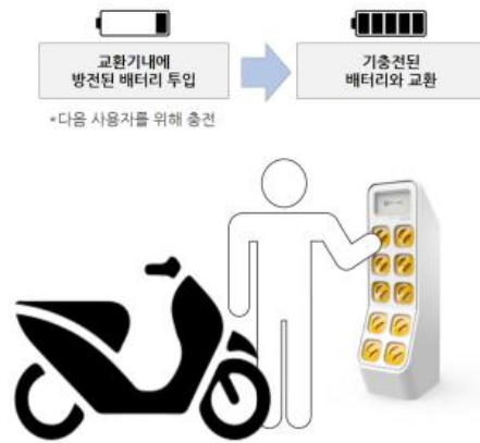
Fig. 2. How to swap the battery
