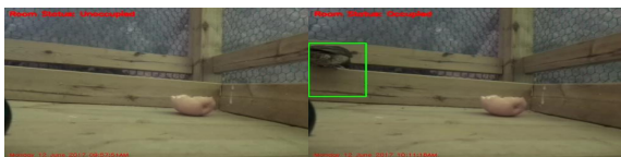
Fig. 2. Camera data of wild bird repeller, the left is the undetected state, and right is the bird detected state.
