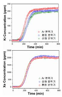
Fig. 2. Breakthrough curves measured at argon, reducing, and oxidizing condition.
