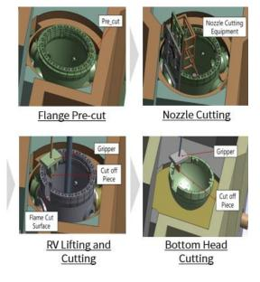
Fig. 2. Process of RV Dismantling.
