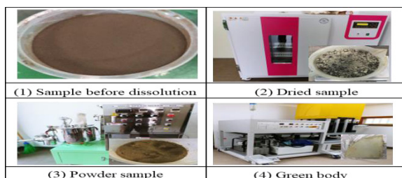
Fig. 1. Process for Manufacturing Powder Sample. The role of additives in the mixed sample is to maintain the state of glass ceramic compound and the shape of structure during the process of heat treatment.
