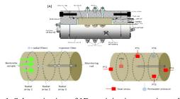
Fig. 1. Schematic view of 1D gas injection experiment [3].
