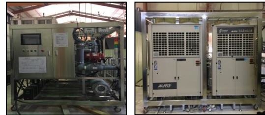
Fig.1. Left: drying skid / right: chiller skid.
