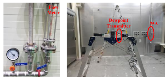
Fig.2. Flow Meter and Dewpoint Transmitter.
