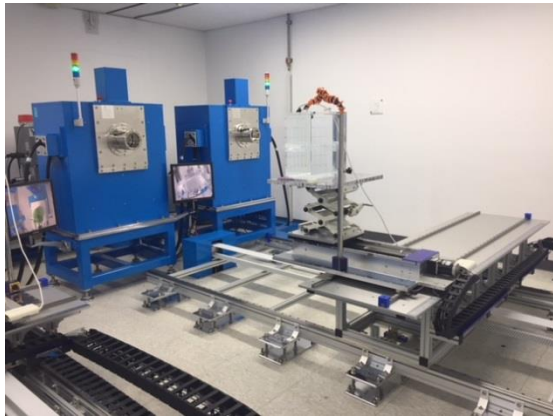
Fig. 1. X-ray generator in KHNP CRI.
