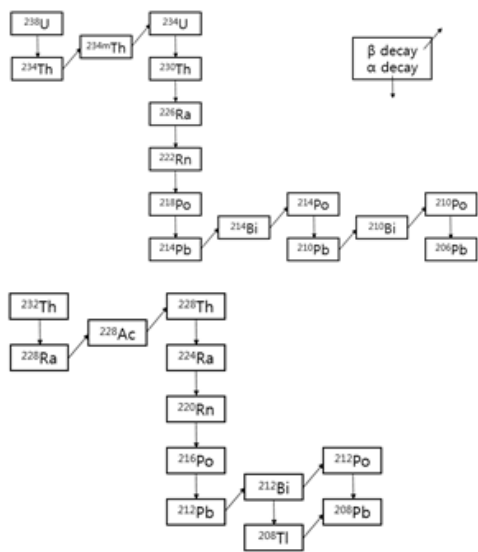
Fig. 2. The decay schemes of uranium and thorium.
