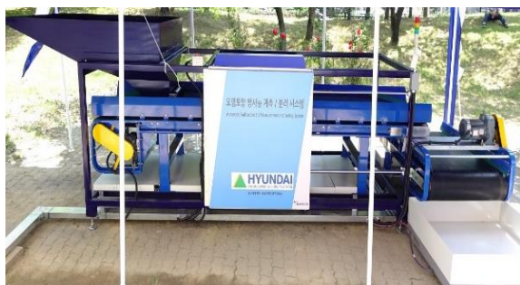
Fig. 4. Real-time measurement and segregation system.
