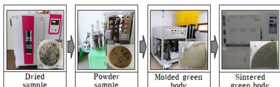
Fig. 1. The process for Manufacturing sintered green body.
