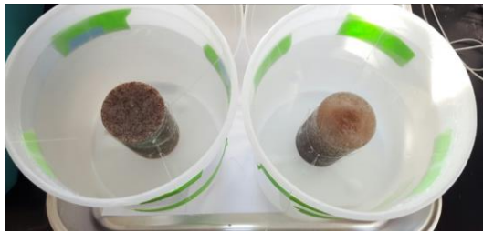
Fig. 2. ANSI/ANS 16.1 test of 19 days.
