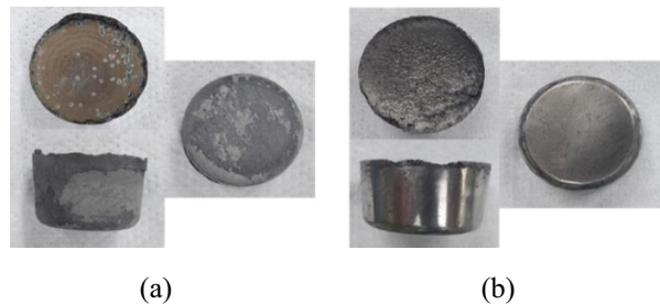
Fig. 1. The surface states of U-10Zr-5RE melt residue in as-cast state (a) and after (b) mechanical treatment.
