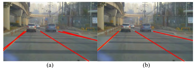
Fig. 8: (a) lines detected, (b) average of lines in each cluster.
