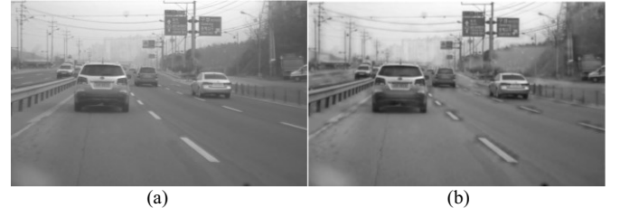
Fig. 3: (a) Lightness channel, (b) contrast enhancement with CLAHE.
